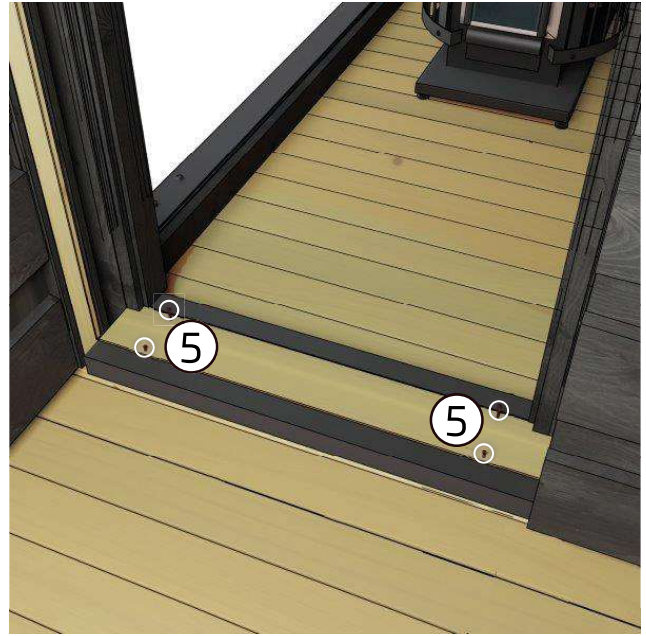
11. Attach the threshold board using screws ( 5 ). The threshold board has pre-drilled holes.
